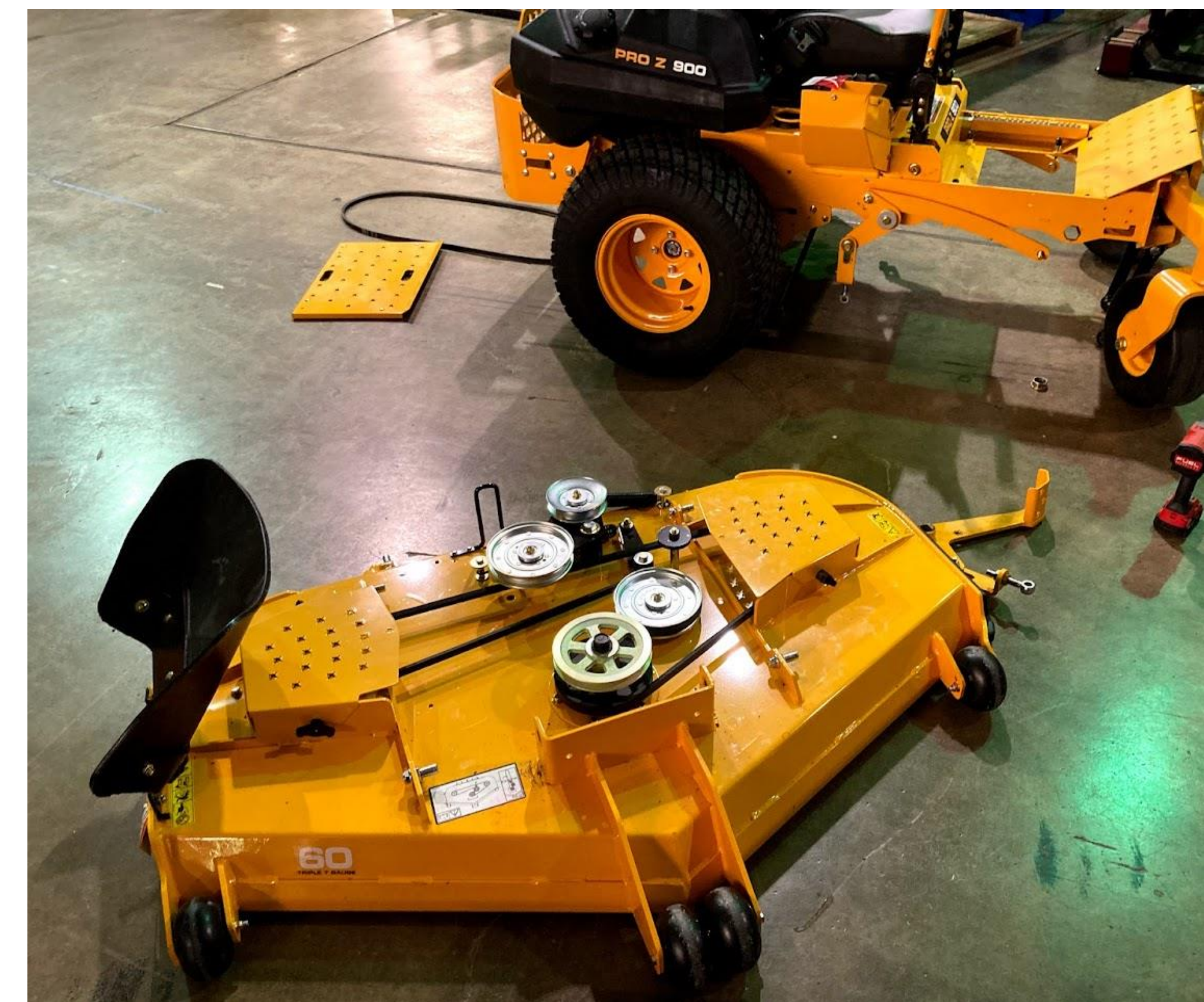
Verifying deck belt replacement procedure in the shop
