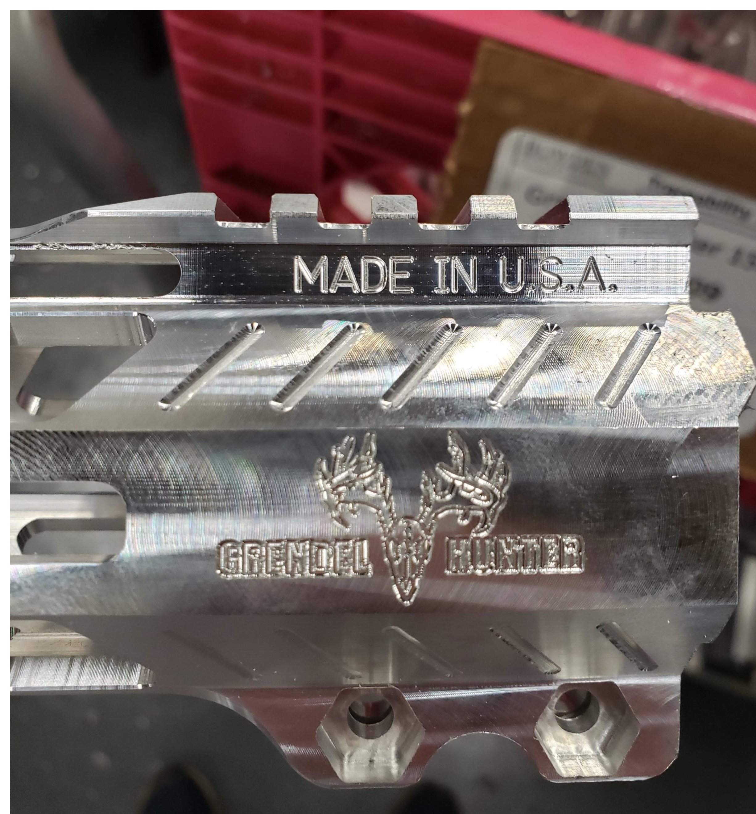
Aluminum part machined on Haas CNC mill
