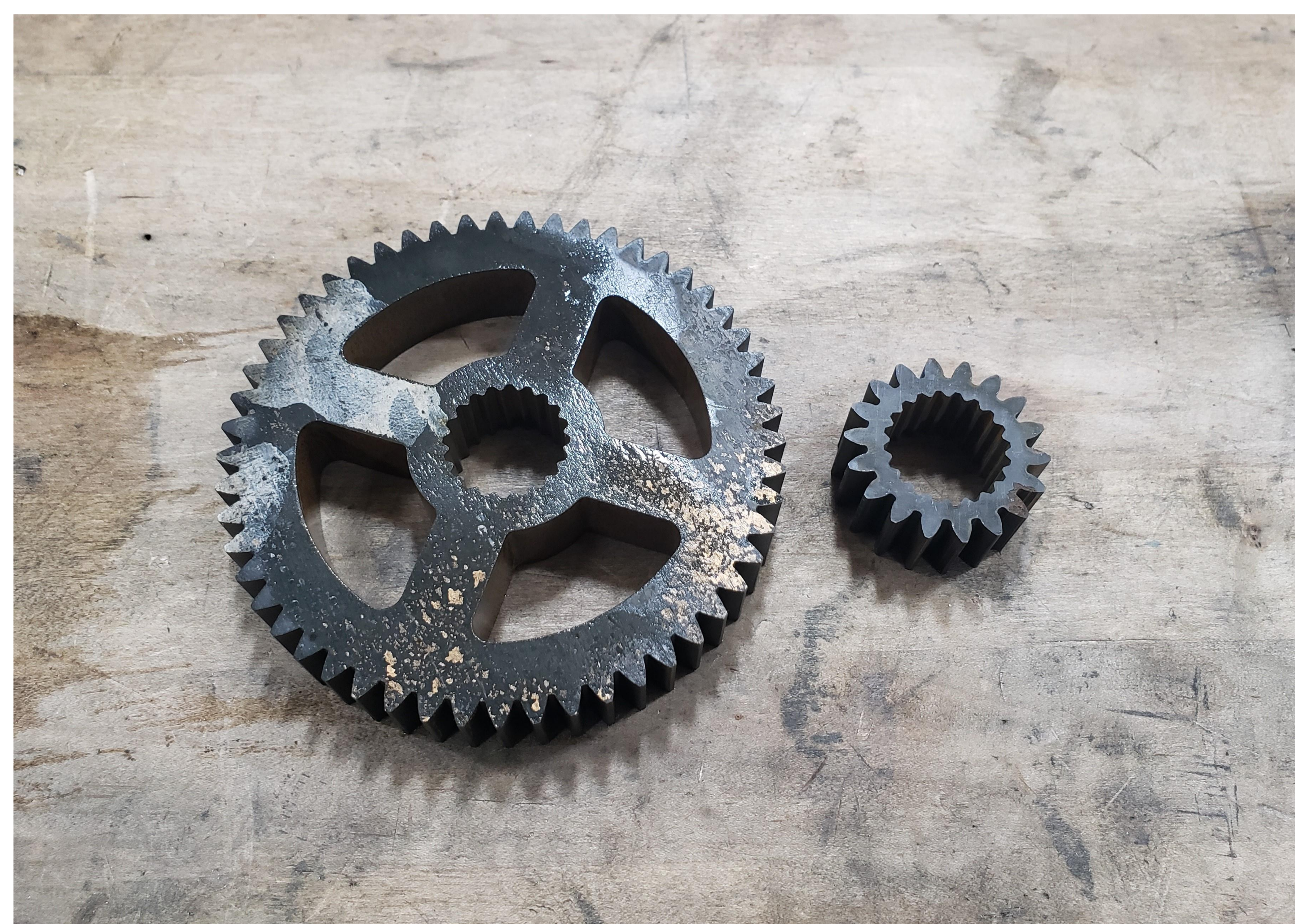
Gears made using wire EDM
