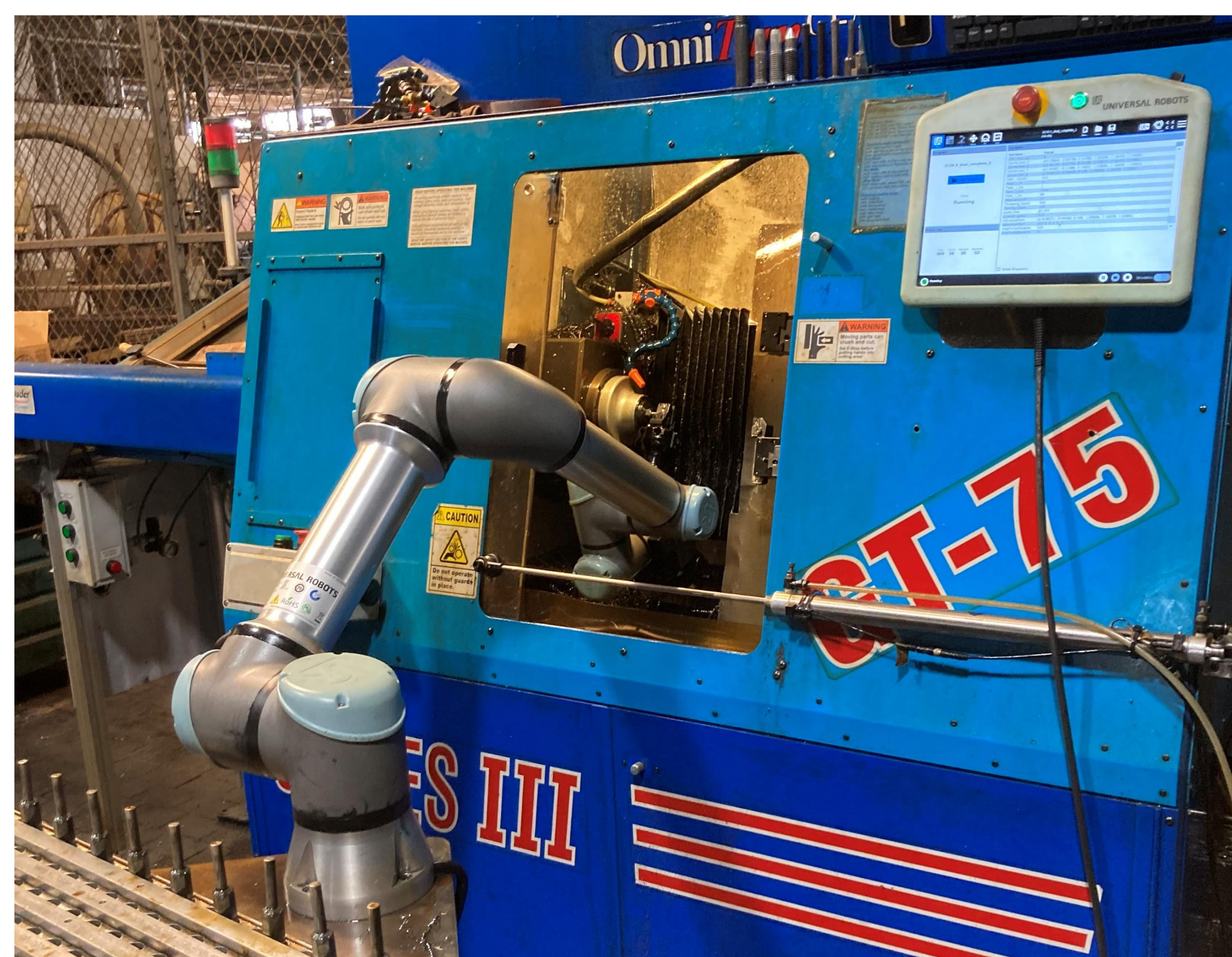
Figure 2. OmniTurn GT-75 with integrated robotic arm
