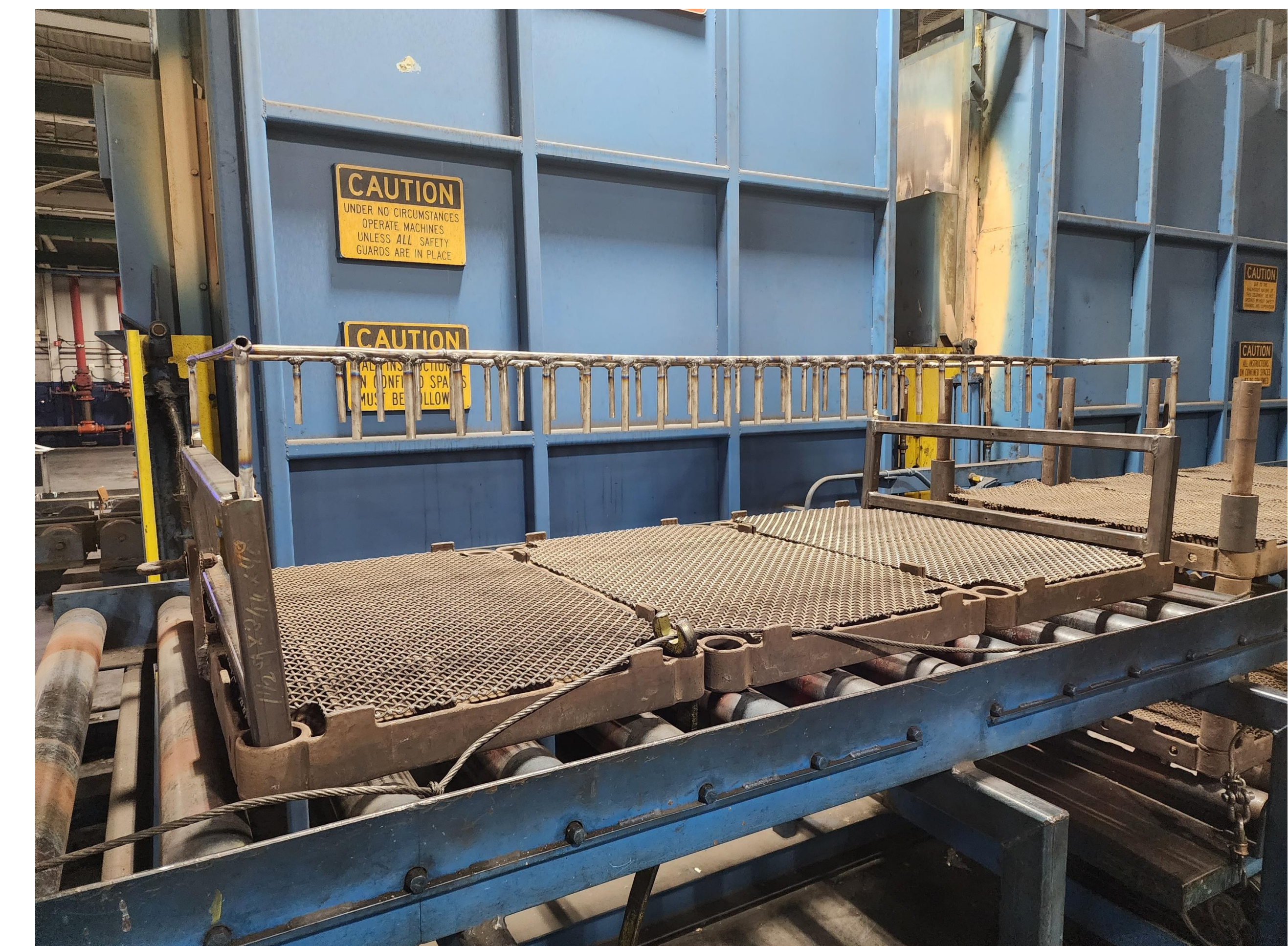
Part spacing rack made from titanium tubing.
