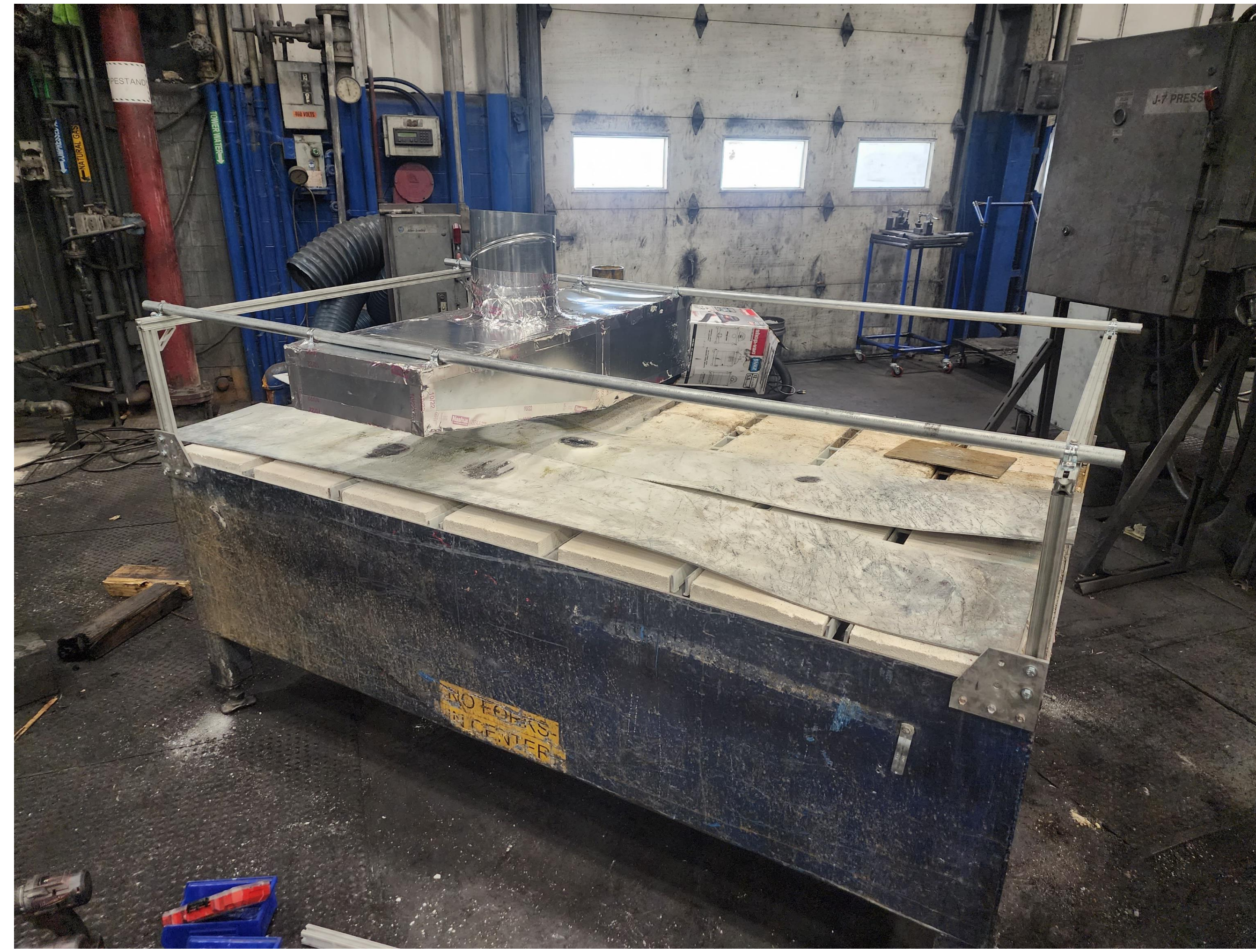
Smoke elimination hood; to be hooked up to a downtorrit system.
