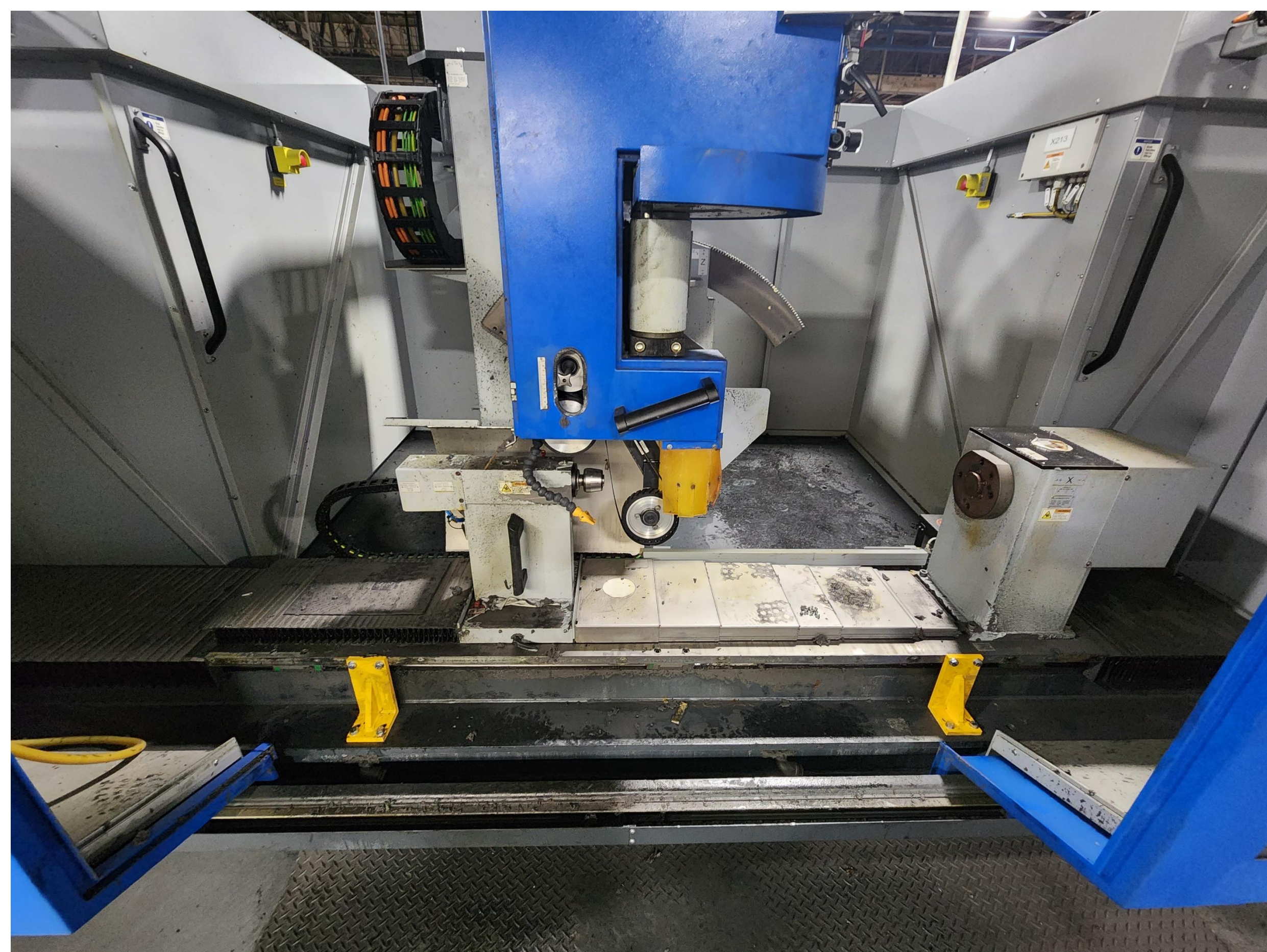
Grinding CNC locked axis and prepared for shipping.
