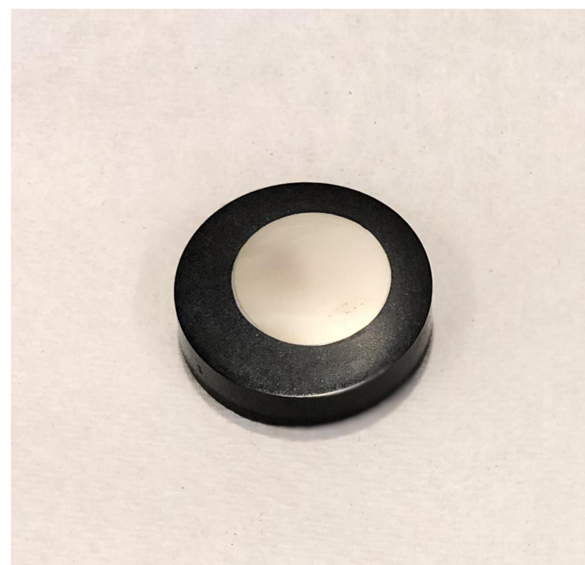
Figure 1. Final Polished Sample of Ni-10TiC
