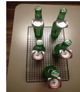
Figure 2: Warming Set-up for Glass Bottles
