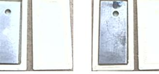
No corrosion seen after 24 hours
