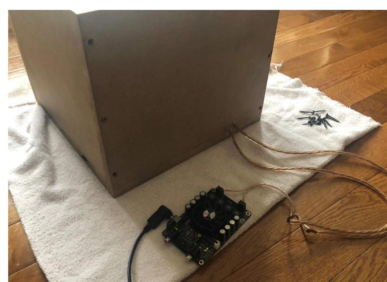
Figures 3 and 4. Shown is our amplifier board to power our speaker along with the attached power supply.
