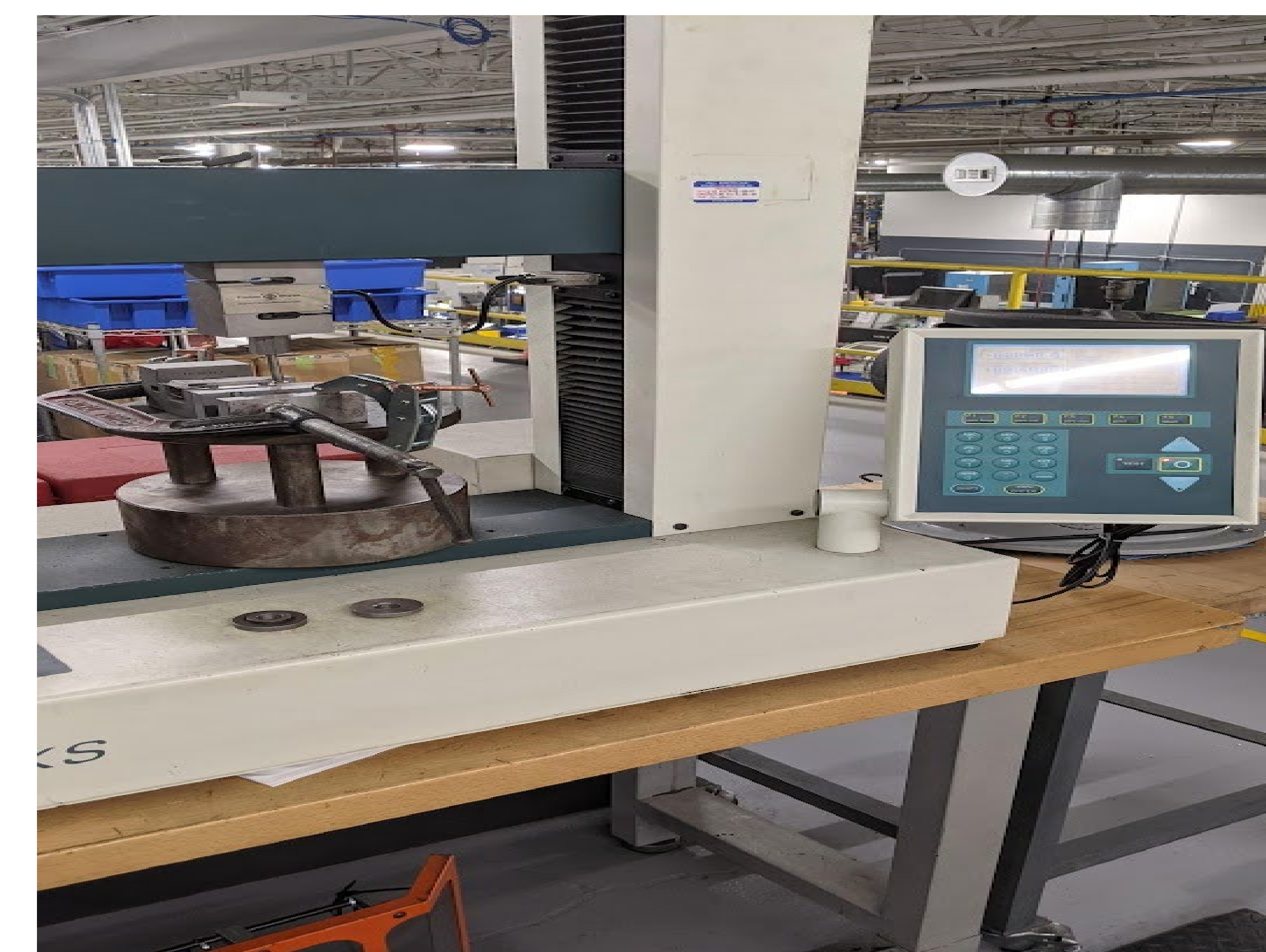
Figure 3. Testing of trigger assembly.
