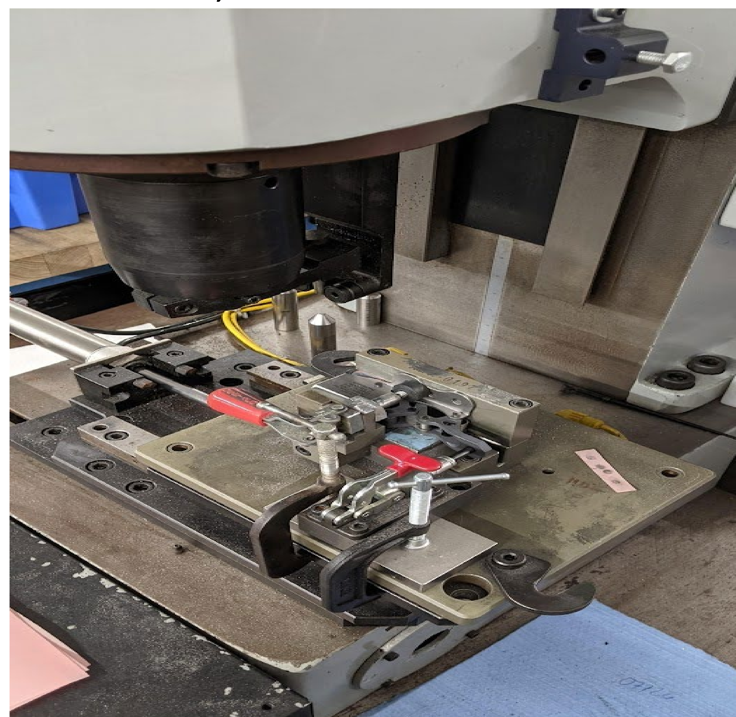
Figure 2. Redesign of riveting fixture.
